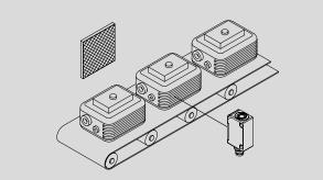
**Checking completeness** The presence of the inserted components must be checked before further production steps.
