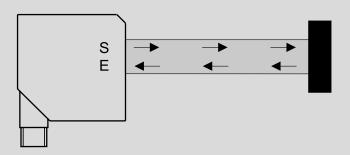
The transmitter and receiver of a diffuse sensor are accommodated in a single housing. The light emitted by the transmitter hits the target object, which reflects the light. This returning light is evaluated by the receiver. The advantage of this method is that no reflector is required.
