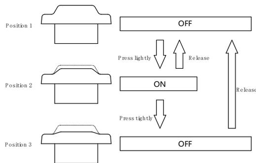
Position 1 and 2. Positions of the enabling switch
