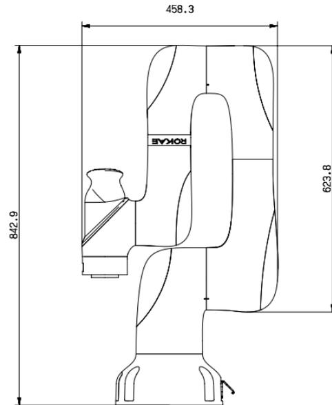
Figure 11. Reference transportation dimensions of the robot
