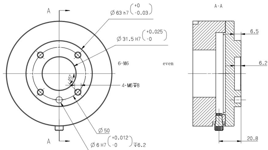
Figure 13. Tool flange installation
