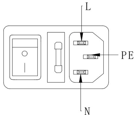
Figure 6-22 Power input interface
