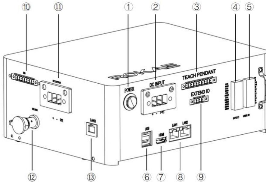
Figure 6-2 Controller interfaces
