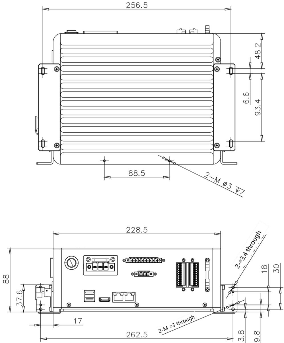
Figure 5-7 Horizontal installation
