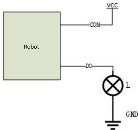
Figure 6-10 PNP output wiring diagram
