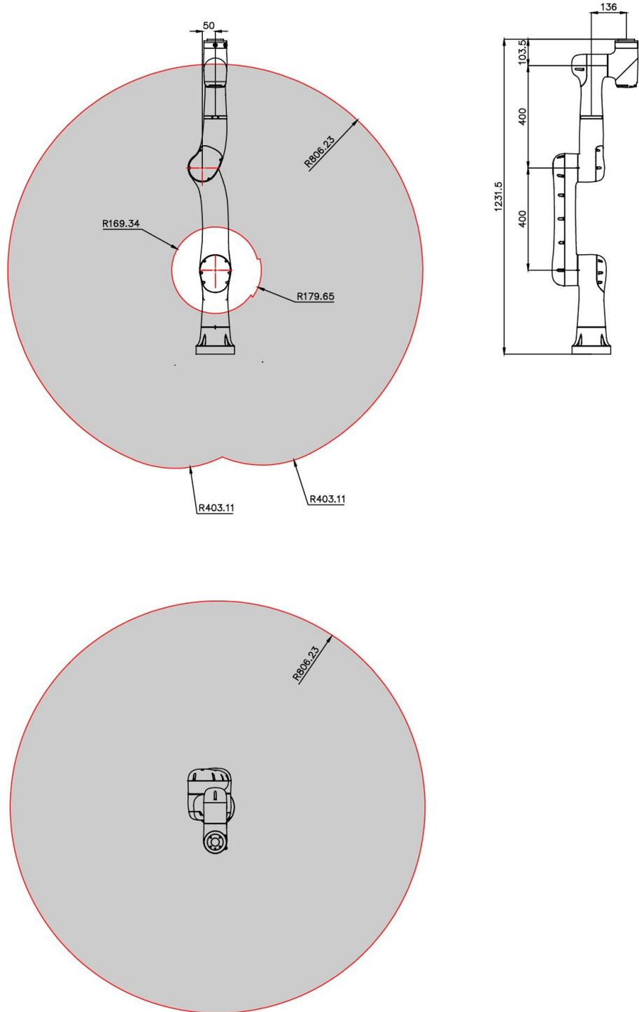
Figure 4-2 Working space of xMate SR4-C
