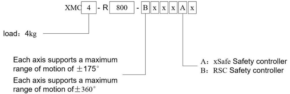
Figure 4-1. The model description of xMate SR4-C
