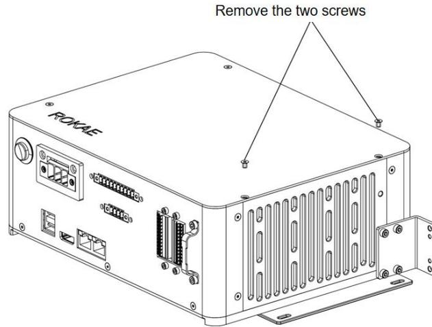
Figure 5-10 Removing screws
