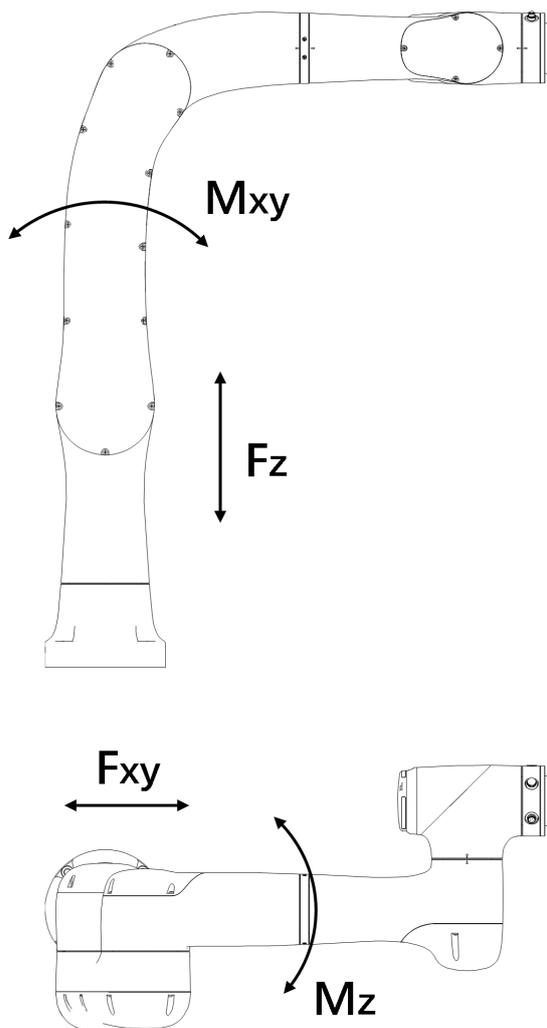
Fig 5-5 Supporting reaction force of the robot
