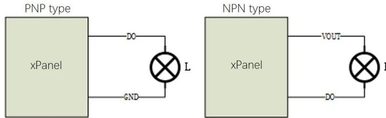
Figure 6-19 End effector output interface
