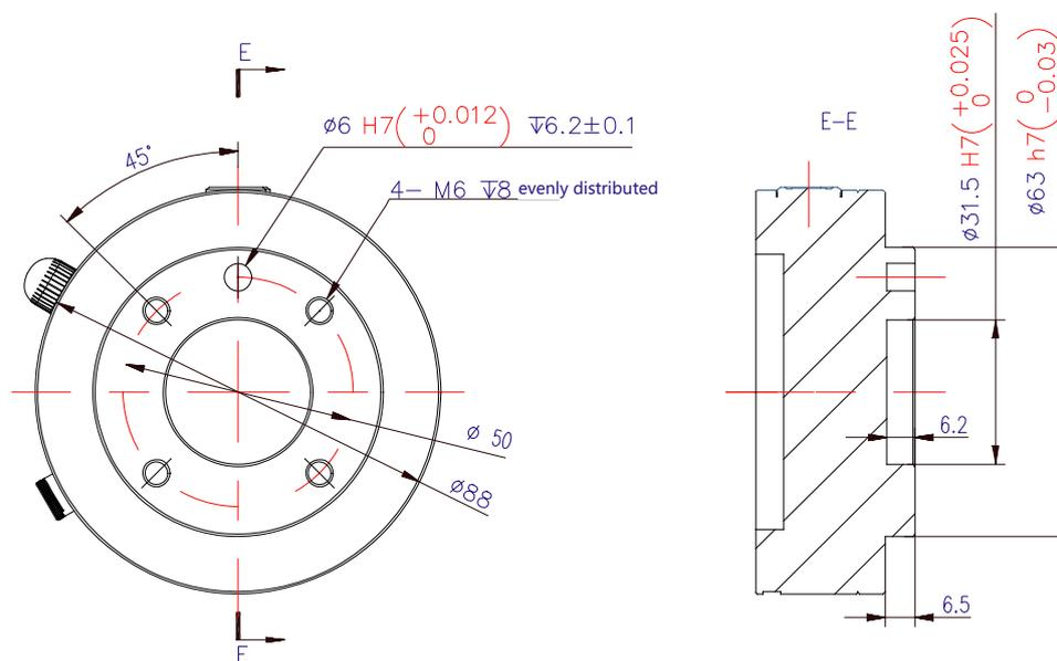
Figure 11. Tool flange installation
