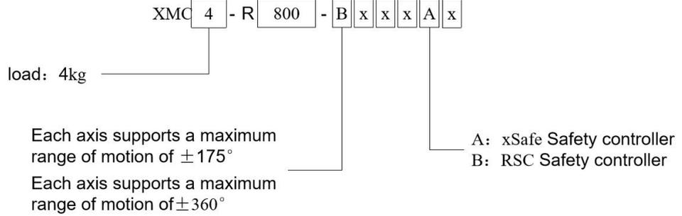
Figure 4-1. The model description of xMate SR4
