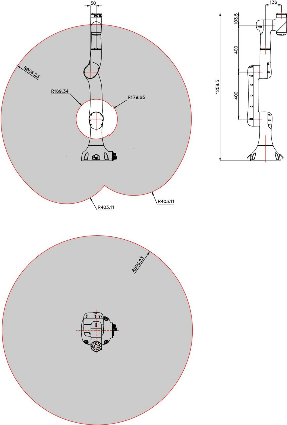
Figure 4-2. The working space of xMate SR4
