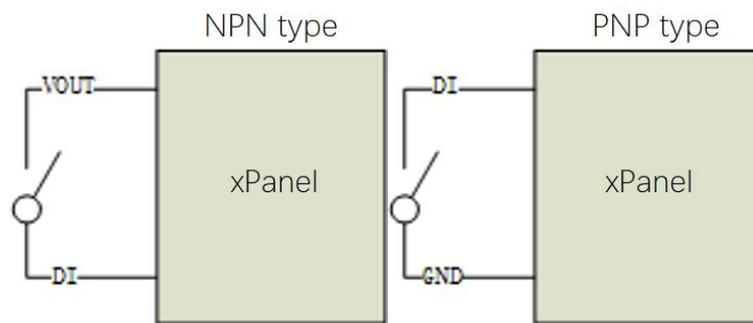
Figure 28. End effector input interface
