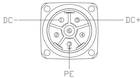
Figure 14. Power supply interface (side view for cables)
