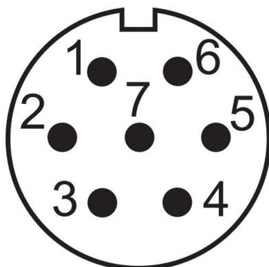
Figure 24. The EtherCAT debug interface
