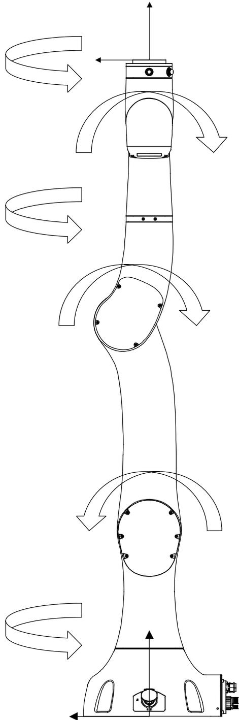
Figure 4. Definitions of robot rotation directions and coordinate systems (for details). The definitions of axis rotation directions and coordinate systems are described below. Base coordinate system: The  $-X$  axis points in the outgoing cable direction of the base, and the  $+Z$  axis in a direction perpendicular to the mounting surface. The  $Y$  axis is determined by the right-hand rule.
