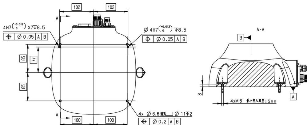
Figure 10. Reference bracket fixing method
