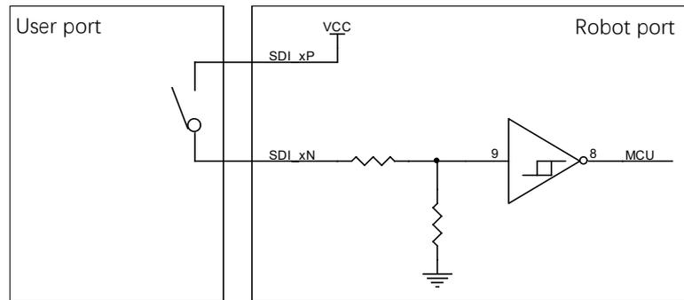
The principle of both loops is the same, and 24 VDC signals are supported. When wiring, if the safety signals 1AP and 1AN, 1BP and 1BN are short-circuited at the same time, the safety input is valid, and if they are open-circuited at the same time, the safety input is invalid, and the others are abnormal state.
