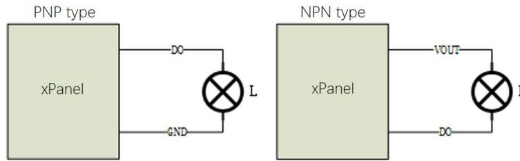
Figure 27. End effector output interface
