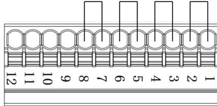
figure xxx Short circuit diagram
