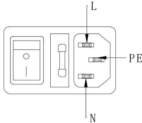
Figure 30. Power input interface
