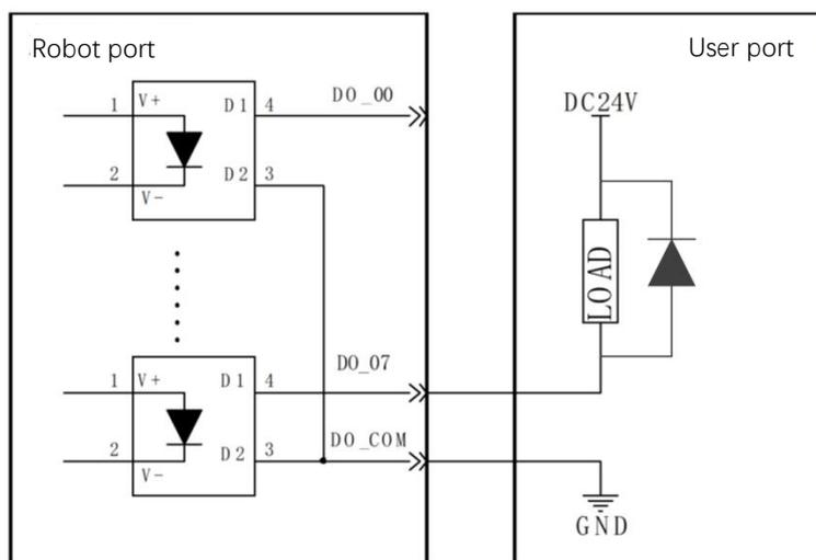
When the output is active high, the DO\_COM (common port) is connected to 24 VDC, as shown below.
