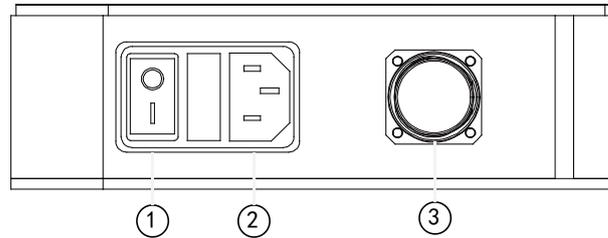
Figure 29. Power adapter interface
