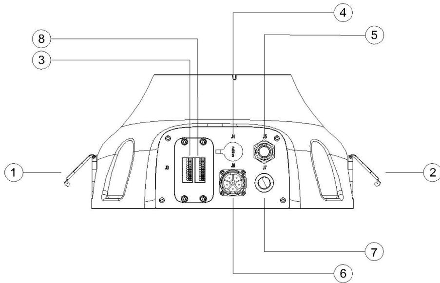
Figure 13. Base interface layout
