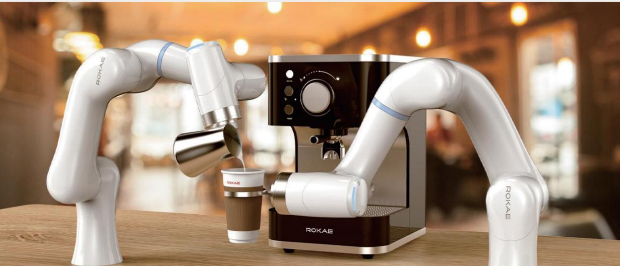
Expanding upon the distinctive features and core advantages of the xMate SR flexible cobot, the **xMate SR-C** takes it a step further by relocating the controller to create an independent controller cabinet. This design caters to more confined base installation environments. Furthermore, the xMate SR-C undergoes a comprehensive upgrade, now supporting a 5 kg payload capacity.
