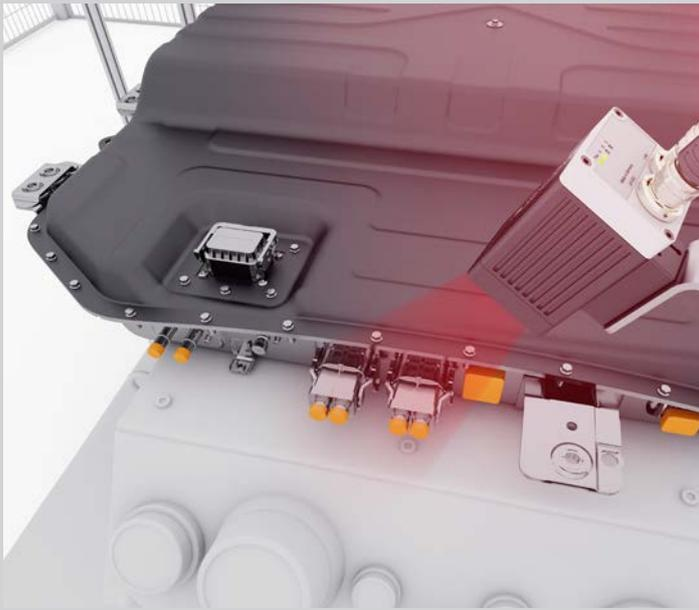
The VISOR® Object in combination with a robot provides the necessary flexibility for inspecting hard-to-see protective caps. Thus, the desired image acquisition for a reliable inspection succeeds. The
