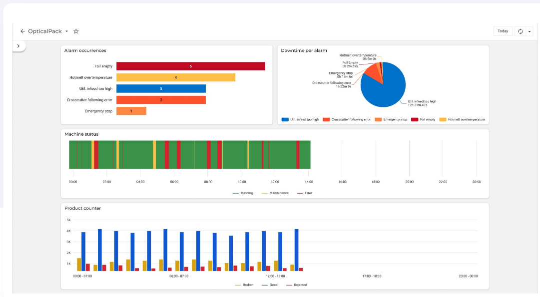
Analysis of downtime with machine status, alarm occurrences, and downtime per alarm.
