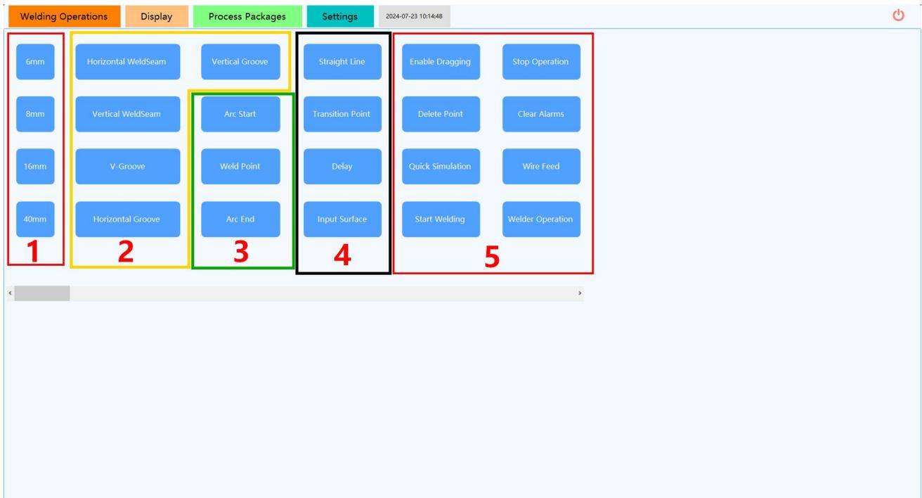
(1) This part is commonly used plate thickness, and the plate thickness value can be customized in the settings.
