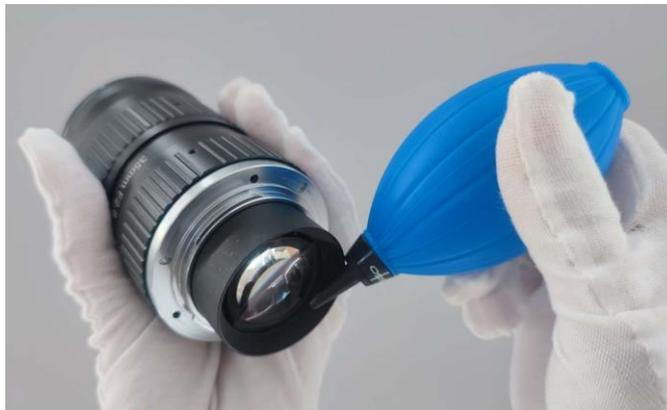
**Figure 2-1 Cleaning by Rubber Dust Air Blower**
