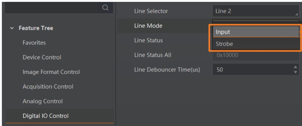
**Figure 9-6 Set Line 2 as Input Signal**
