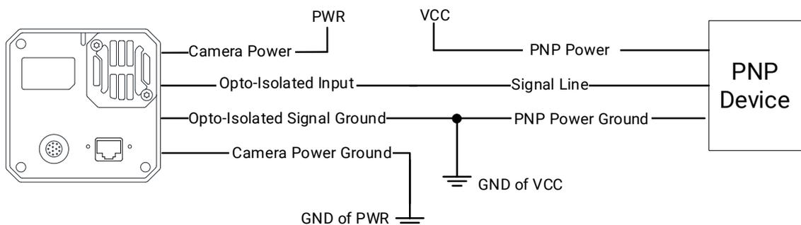
Figure 8-8 Input Signal Connects to PNP Device
