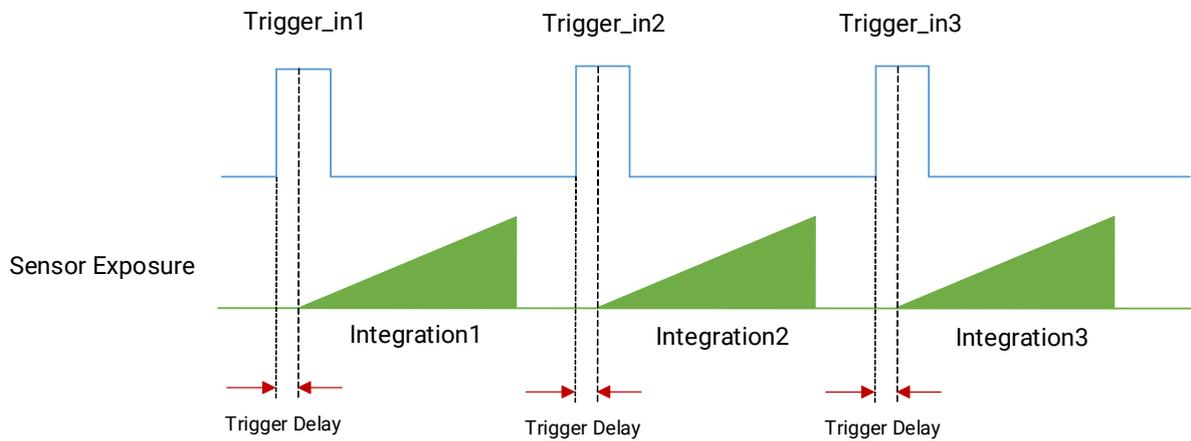
Figure 9-13 Sequence Diagram of Trigger Delay
