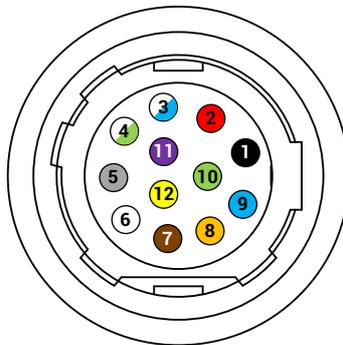
**Figure 4-4 12-Pin P10 Connector for Device with Fiber Port**
