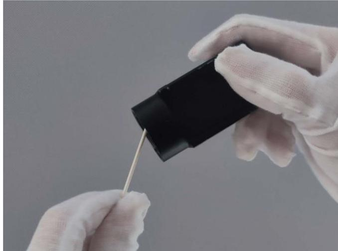
**Figure 2-2 Contact Cleaning**
