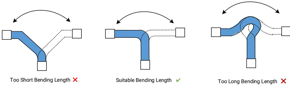
**Figure 6-4 Suitable Bending Length**
