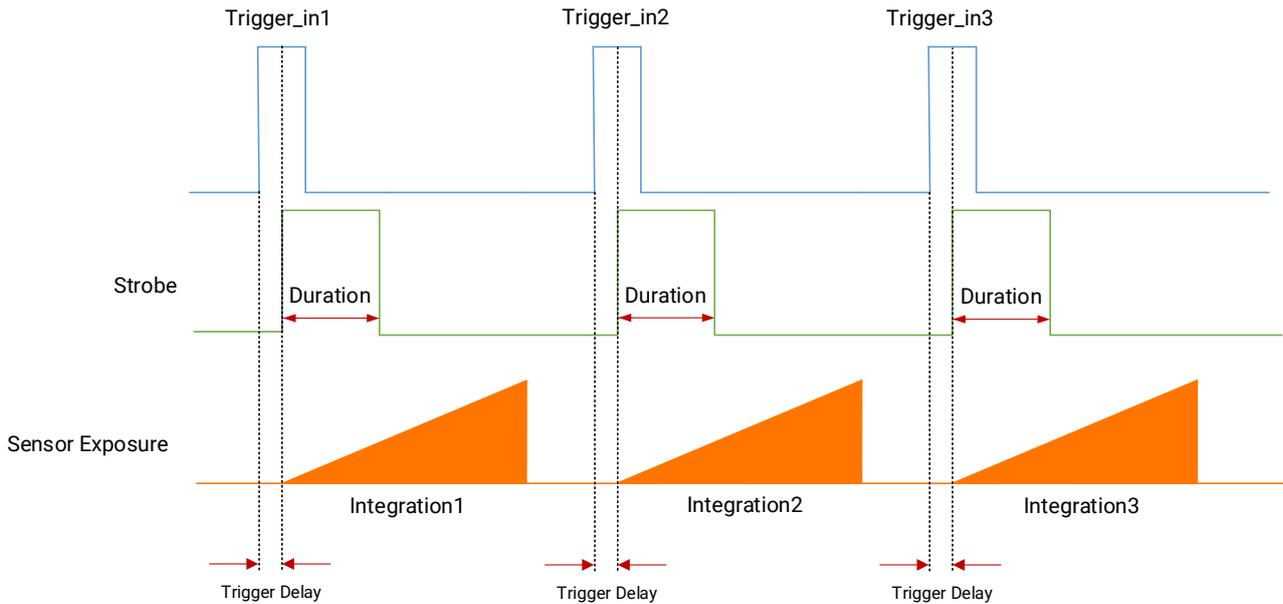
**Figure 9-27 Sequence Diagram of Strobe Line Duration**
