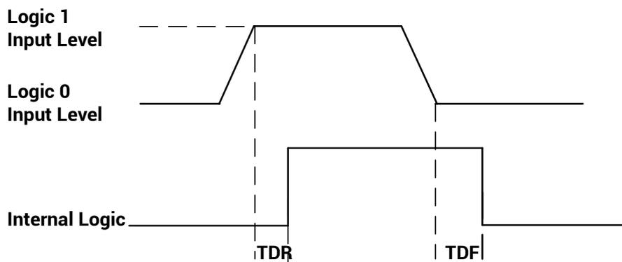
Figure 8-2 Input Logic Level
