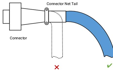
**Figure 6-6 Assemble Connector**
