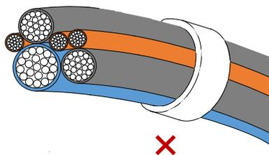
**Figure 6-7 Improper Binding**
