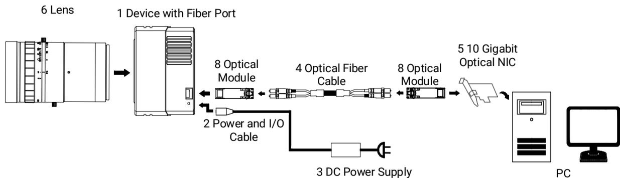
**Figure 7-3 Topology Diagram of Device with Fiber Port**
