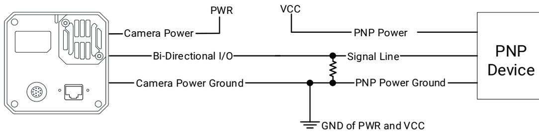
**Figure 8-13 Input Signal Connects to PNP Device**
