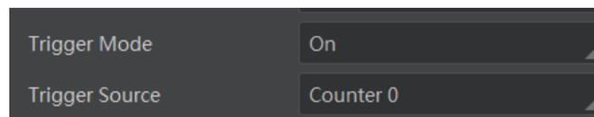
**Figure 9-7 Set and Execute Counter Trigger**
