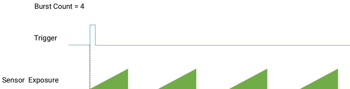
Figure 9-11 Sequence Diagram of Acquisition Burst Frame Count
