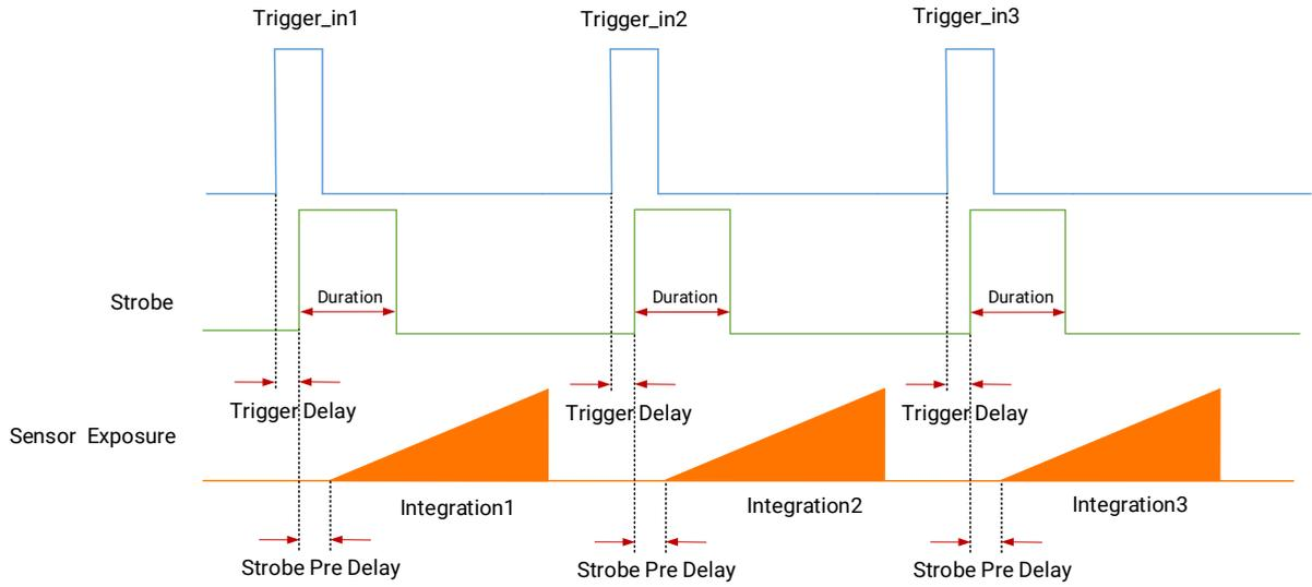
**Figure 9-31 Sequence Diagram of Strobe Pre Line Delay**
