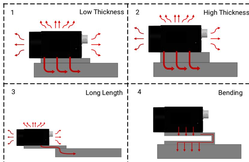
**Figure 5-4 Heat Conduction Path of Different Installation Methods**
