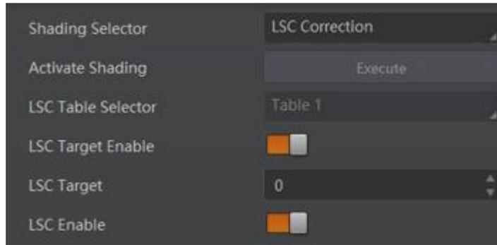
**Figure 13-11 Correct Image via Setting Parameters**
