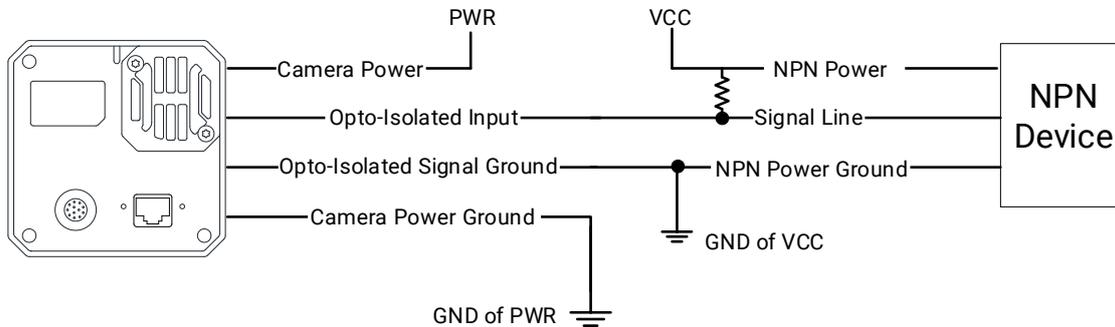
**Figure 8-9 Input Signal Connects to NPN Device**
