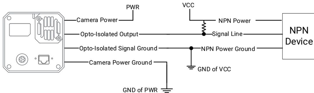
Figure 8-12 Output Signal Connects to NPN Device
