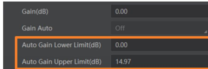
Figure 12-27 Set Gain under Once or Continuous Mode
