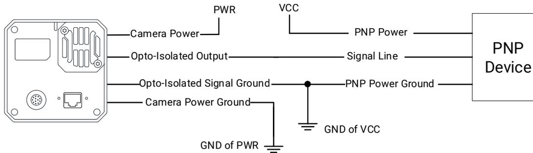
Figure 8-11 Output Signal Connects to PNP Device
