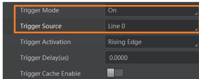
**Figure 9-5 Set Line 0 or Line 2 as Input Signal**
