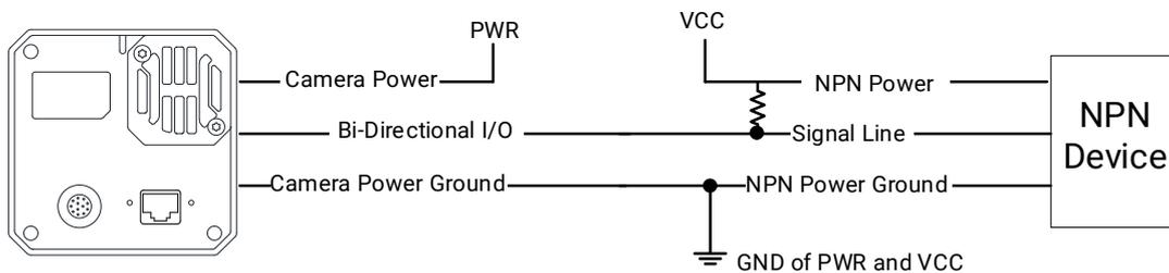
Figure 8-17 Output Signal Connects to NPN Device
