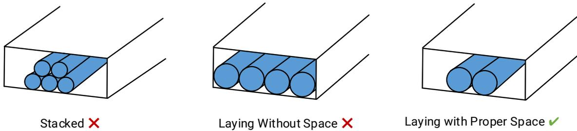
**Figure 6-1 Cable Laying**
