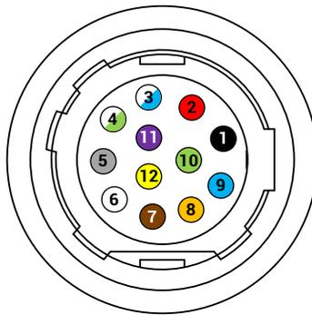
Figure 4-3 12-Pin P10 Connector for Device with RJ45 Network Interface
