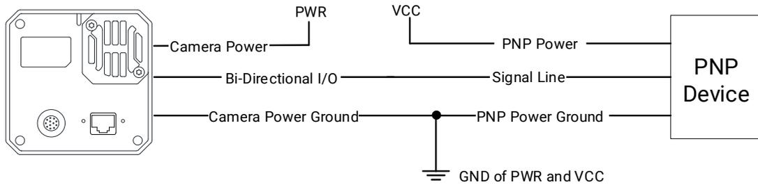
Figure 8-16 Output Signal Connects to PNP Device
