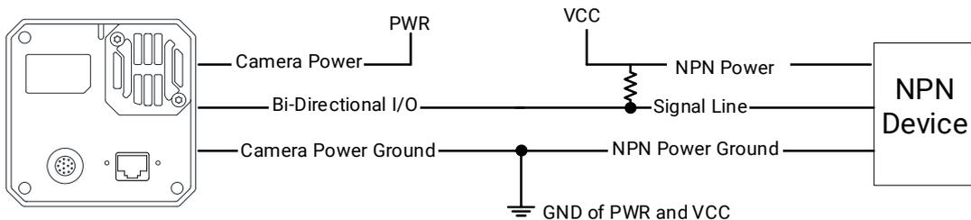
**Figure 8-14 Input Signal Connects to NPN Device**
