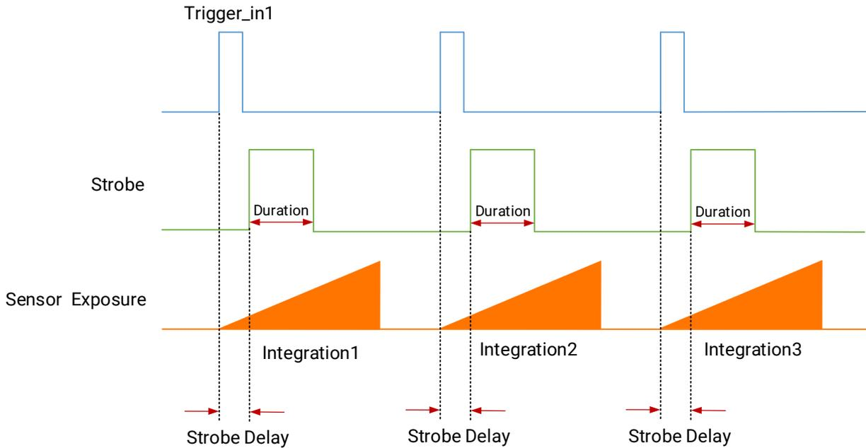
**Figure 9-29 Sequence Diagram of Strobe Line Delay**
