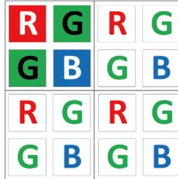
**Figure 12-14 Binning Horizontal 2 and Binning Vertical 2**
