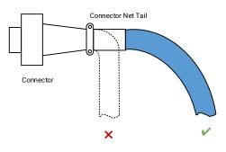
Figure 6-6 Assemble Connector
