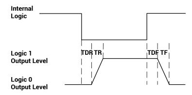
Figure 8-7 Output Logic Level
