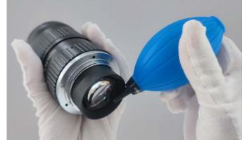
Figure 2-1 Cleaning by Rubber Dust Air Blower
