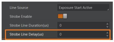
Figure 9-28 Set Strobe Line Delay
