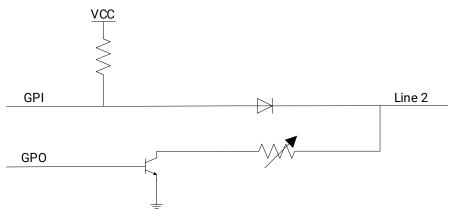
Figure 8-5 Internal Circuit of Bi-Directional Signal
