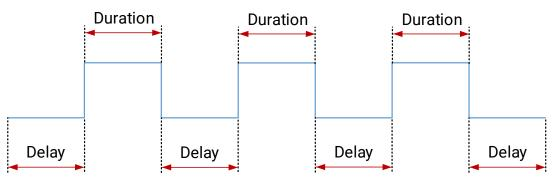
Figure 9-25 Sequence Diagram of Timer Active
