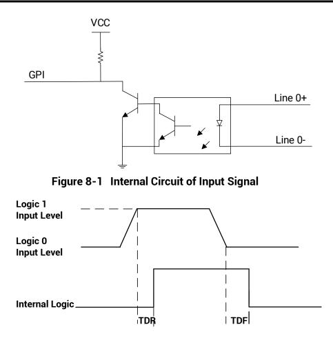
Figure 8-2 Input Logic Level
