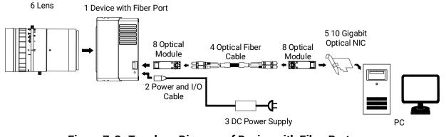
Figure 7-3 Topology Diagram of Device with Fiber Port
