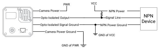
Figure 8-12 Output Signal Connects to NPN Device
