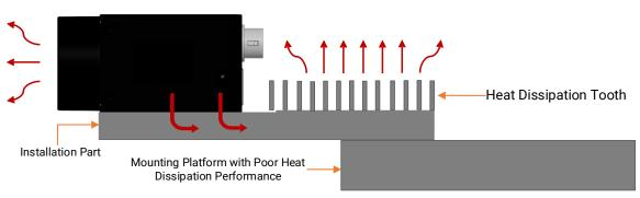
Figure 5-5 Add Heat Dissipation Tooth
