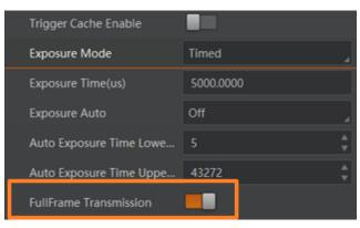
Figure 11-3 Set Full Frame Transmission
