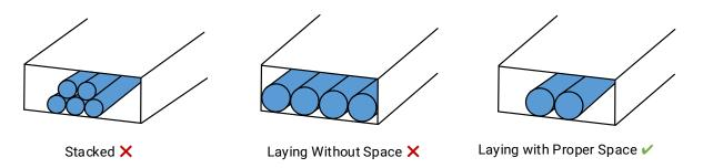
Figure 6-1 Cable Laying
