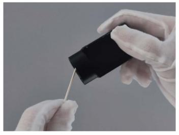
Figure 2-2 Contact Cleaning
