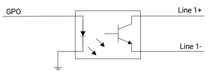
Figure 8-3 Internal Circuit of Output Signal
