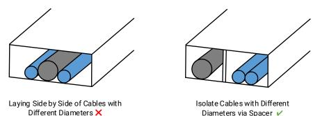
Figure 6-2 Isolated via Spacer
