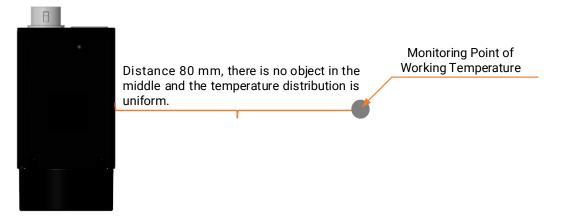
Figure 5-1 Monitoring Point of Working Temperature
