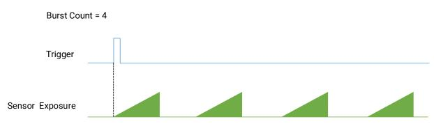
Figure 9-11 Sequence Diagram of Acquisition Burst Frame Count
