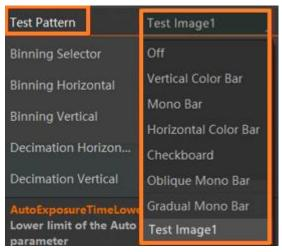
Figure 12-11 Set Test Pattern
