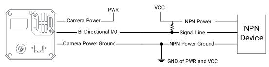
Figure 8-17 Output Signal Connects to NPN Device
