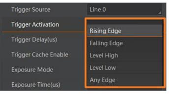
Figure 9-18 Set Trigger Activation
