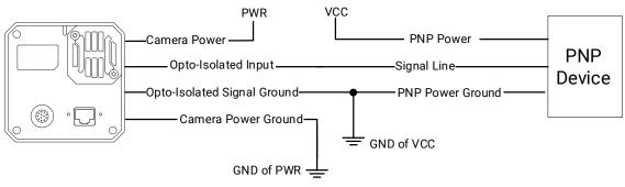
Figure 8-8 Input Signal Connects to PNP Device
