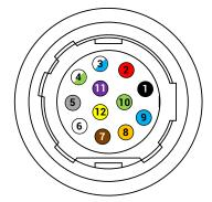
Figure 4-3 12-Pin P10 Connector for Device with RJ45 Network Interface
