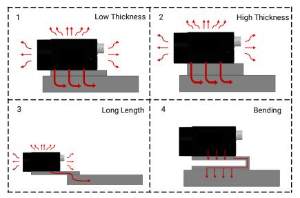
Figure 5-4 Heat Conduction Path of Different Installation Methods
