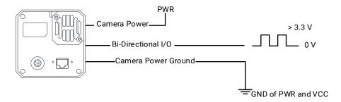
Figure 8-15 Input Signal Connects to Switch
