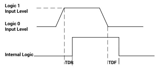
Figure 8-6 Input Logic Level
