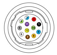
Figure 4-4 12-Pin P10 Connector for Device with Fiber Port
