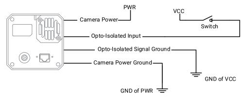
Figure 8-10 Input Signal Connects to Switch
