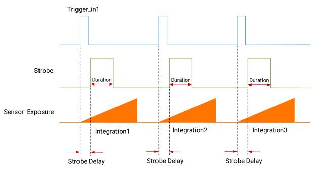
Figure 9-29 Sequence Diagram of Strobe Line Delay
