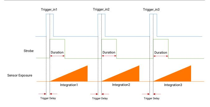
Figure 9-27 Sequence Diagram of Strobe Line Duration
