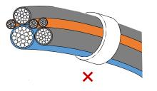
Figure 6-7 Improper Binding
