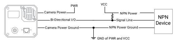
Figure 8-14 Input Signal Connects to NPN Device
