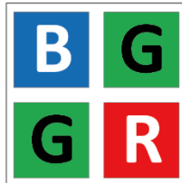
Figure 12-9 Bayer BG Pixel Pattern
