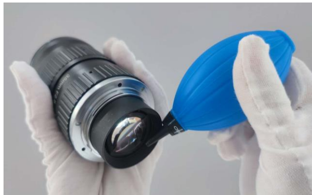
Figure 2-1 Cleaning by Rubber Dust Air Blower
