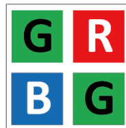
Figure 12-7 Bayer GR Pixel Pattern
