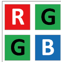
Figure 12-10 Bayer RG Pixel Pattern
