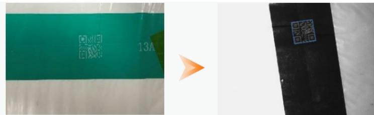
After the battery cells are wound/stacked, the termination tape is usually applied for the insulation fixation of the termination part of the cells, and the quality of the cells is traced through the QR code, and the code reading rate of this solution reaches more than 99.99%.
