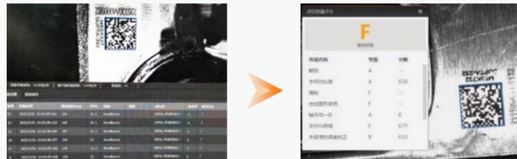
Identify the DM code on the top cover piece of lithium battery, metal reflective material. ID5050 smart code reader with polarized lens hood to overcome reflections, DM code stable identification, read the code level close, read the code rate of 99.99% or more.
