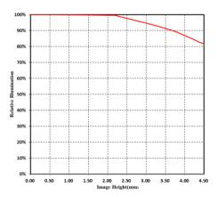
Note: The above curves are the simulate results based on F2.4,  $\beta$ =-0.029, WD=400 mm.
