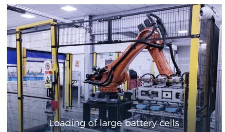
Loading of large battery cells
