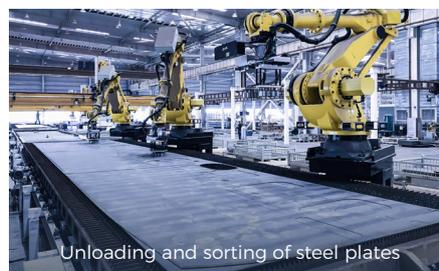
Unloading and sorting of steel plates
