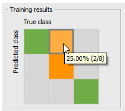
Fig. 221: Training results - 25% detected incorrectly
