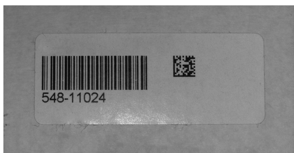
Fig. 283: Comparison of DataMatrix code and barcode
