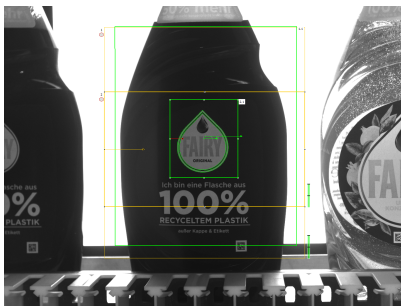
Fig. 278: Case 1: Label correctly applied
