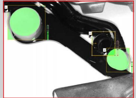
software provides the function to determine the presence of the caps based on a unique grey value and, if necessary, to check their position. To check different types of caps with the same hardware, the vision sensor offers the possibility to change jobs. The duration of the image evaluation is only a few milliseconds, so that a protective cap inspection is possible in passing.
