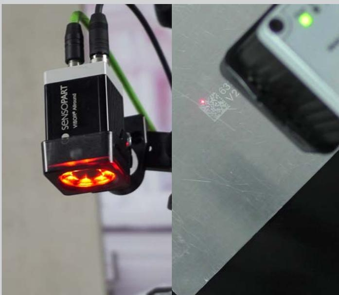
Trouble with shiny surfaces? No problem! This is where a polarizing filter kicks in. With this helpful accessory, details can be detected regardless of the reflectivity of the surface. The switchable version with 50% coverage of the LEDs can reliably detect the object even if the texture of the surface varies without changing the filter. Installation is very easy by simply „clicking“ it onto the VISOR®.
