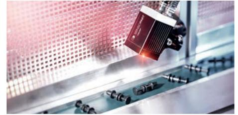
Presence, completeness, measurement, position check, color, reading of barcodes, data codes, text, multi-shot
