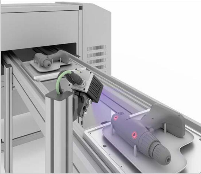
Often screws are sealed by a fluorescent ink to be able to check whether they have been opened or if the product is still sealed. It's done with invisible ink so that the end customer does not see the marking. The presence of this fluorescent ink can be checked by the VISOR® Allround UV. For the evaluation of the luminescent markings, the user has the same extensive detection tools at his disposal as the classic illumination variants (white, red, infrared) of the VISOR® Allround series.
