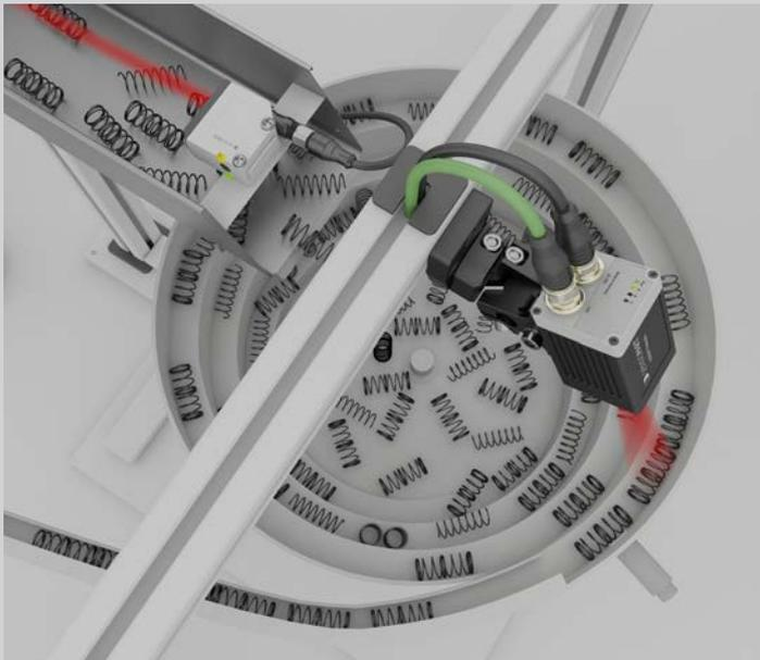
With the classification detector of the VISOR® Object AI, even very similar looking springs are reliably distinguished and correctly fed to the machine. By assigning only a few examples of each class, the classifier automatically learns to distinguish the different types.
