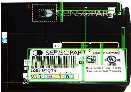
**VISOR® Allround – Object detection in color plus identification united in one device**
