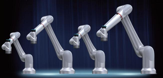
Model CR7 Payload 7 kg Reach 988 mm Model CR12 Payload 12 kg Reach 1,434 mm Model CR18 Payload 18 kg Reach 1,062 mm Model CR20 Payload 20 kg Reach 1,798 mm
