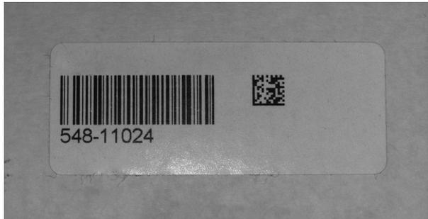
**Fig. 265:** Comparison of DataMatrix code and barcode
