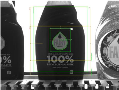
Fig. 260: Case 1: Label correctly applied
