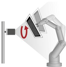
The "Base-Eye calibration (Robotics)" calibration method is used to determine the reference from Camera coordinate system to the robot base (position and orientation) when the vision VISOR® sensor is mounted stationary.
