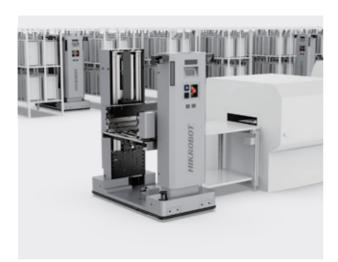
Docking with upper and lower plate stackers & PCB frame
