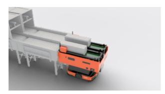
Square crystal silicon ingot carrying in photovoltaics industry
