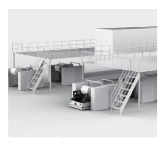
The loading of coating (replace the empty shaft with the loaded rob)
